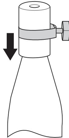
Turn the setscrew to the left, if the diameter of the clip is too small, in order to increase it. Push the adapter as far, as it rests shortly at the bottle neck.
